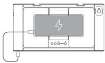
**Note:** Turn on the wireless charging mode but do not clip the smartphone onto the rig for wireless charging, it can still be wired charged.
