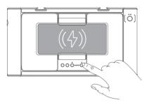
**Wired Charging:** Turn on the device, connect the smartphone to the USB-A port with the USB-A charging cable to charge it.
